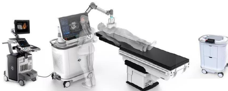
Figure 1: The four-component Edison system. From left to right: a) diagnostic imaging source, b) the Edison System transducer, c) treatment head and d) fluidics cart to create the coupling medium.
